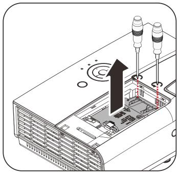
Reverse steps 1 to 6 to install the new lamp module.
